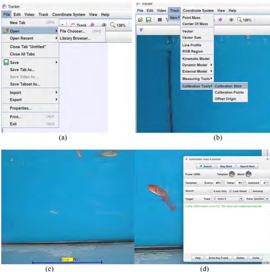
Fig. 2. The process of using the tracker program for the detection of behavioural response in Nile tilapia, *Oreochromis niloticus* (a) select the video for analysis, (b) use a calibration stick, (c) draw a line and set the distance (in this study 0.10 m) and (d) press the search button to capture the velocity of the fish.
