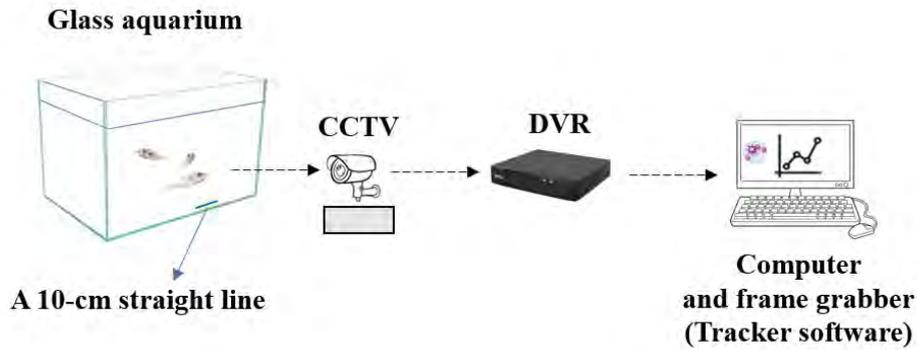
Fig. 1. System overview of posture tracking for fish behavioural monitoring. Closed-circuit television images of fish from the glass aquarium were transmitted to the digital video recorder. Image analysis tracker software analysed fish movement and displayed the result via a user interface in the program. Note: A 10-cm straight line was a marker to capture the fish swimming velocity.
