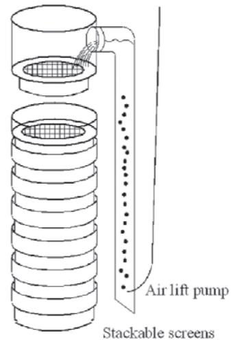
Fig. 1: Screen and stack arrangement used to hold spat and juveniles
