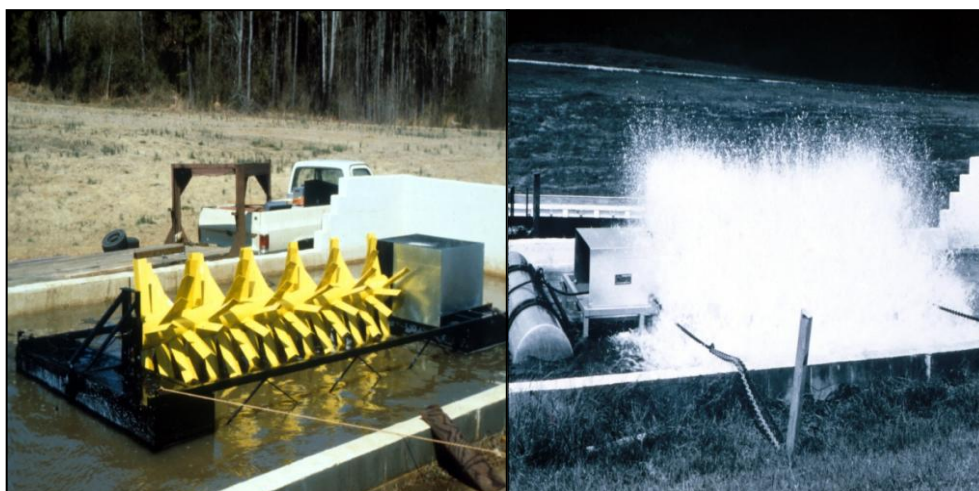
Fig. 4. Floating electric paddlewheel aerator used in channel catfish farming in the United States.
