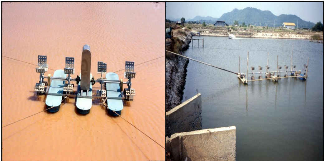
Fig. 3. Asian-style paddlewheel aerators. Left: motor attached to floating frame. Right: motor positioned on the bank and connected to the floating paddlewheel by drive shaft.
